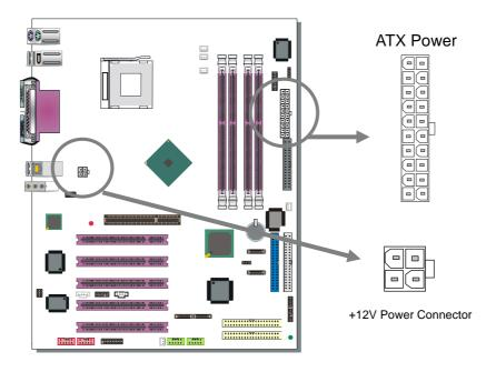
Note 1: The presence of the +12V power connector indicates that a power supply is ATX12V; the absence of the +12Vpower connector indicates that a supply is ATX.
